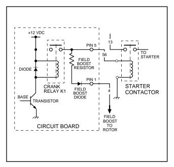
Figure 2. Field Boost Circuit Schematic
